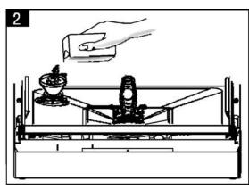
Remove the basket and then unscrew and remove the cap from the salt container.
